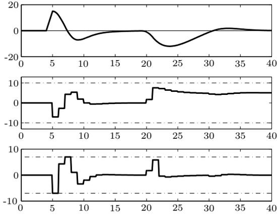
Fig. 2. NMSS/MPC applied to the double integrator plant. Top subplot: reference level and output. Middle subplot: control input (solid trace) and constraints (dash-dot); Lower subplot: input rate-of-change (solid) and constraints (dash-dot).
