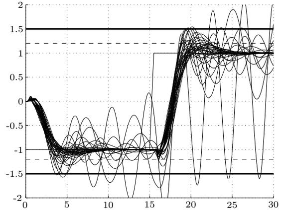
Fig. 4. Robustness test of the IFAC '93 benchmark system for the NMSS/MPC controller based on differenced input and output variables (Wang and Young, 2005)
