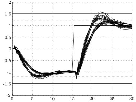
Fig. 3. Robustness test of the IFAC '93 benchmark system for the NMSS/MPC controller with an explicit integral-of-error state variable.
