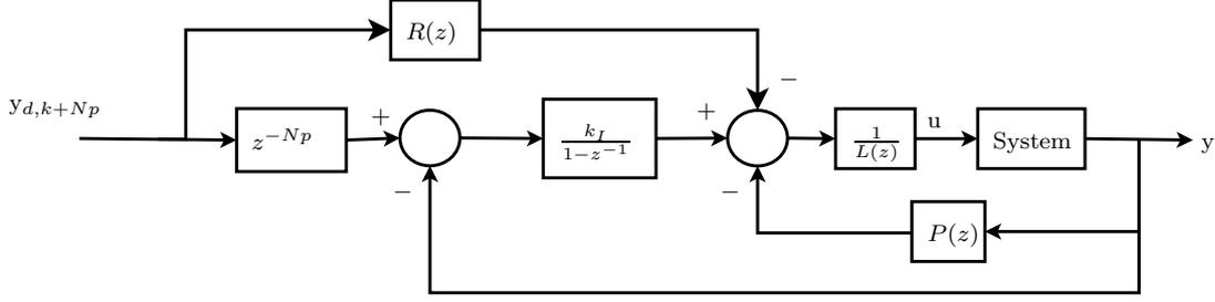
Fig. 1. Proposed MPC in block diagram form.
