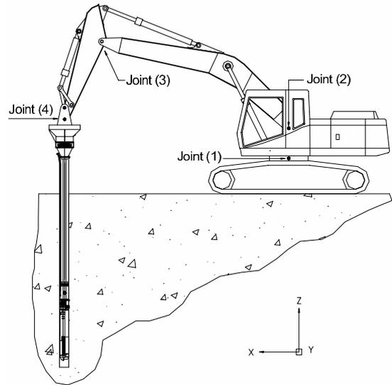
Fig. 1. Two-arm manipulator with vibro-lance.
