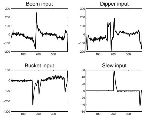
Fig. 3. Scaled input voltages for the experiment in Fig. 2. Positive inputs imply raising the arm or bucket, while negative voltages reverse the direction of movement.
