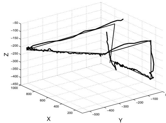
Fig. 4. Resolved position of the end-effector for the experiment in Fig. 2, represented by the planar horizontal and vertical displacements (X and Z), together with the slew (Y), with the set-point shown as straight lines (mm).
