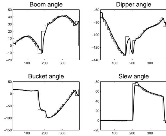
Fig. 2. Implementation results for the laboratory excavator in sand, showing the four joint angles (degrees) and respective set-points, all plotted against sample number.
