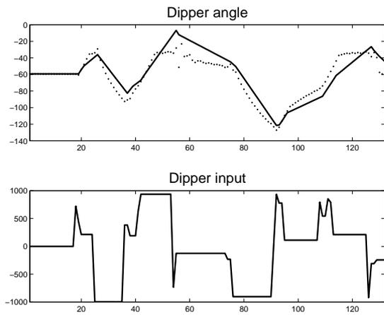
Fig. 5. Open-loop experiment for the vibro-lance being moved in air. Top subplot: SDP model response and experimental data (dots) for the dipper angle. Bottom subplot: scaled voltage.
