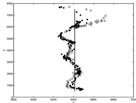
Fig. 6. Implementation experiment for the vibro-lance being lowered in air, showing the resolved position of the end effector, represented by the horizontal and vertical displacements (mm). Nonlinear SDP-PIP control (thick crosses) is compared with linear PIP (circles) and horizontal set point (solid).
