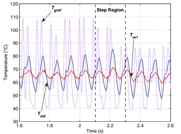
Fig. 5. Temperature variation of TTP under a step change in gas velocity.
