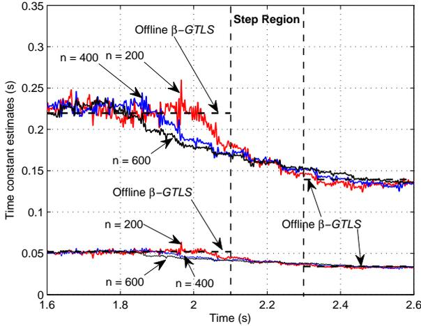
Fig. 7. Time constant estimates using  $\beta$ -GTSL sliding window algorithm with varying sized data windows.
