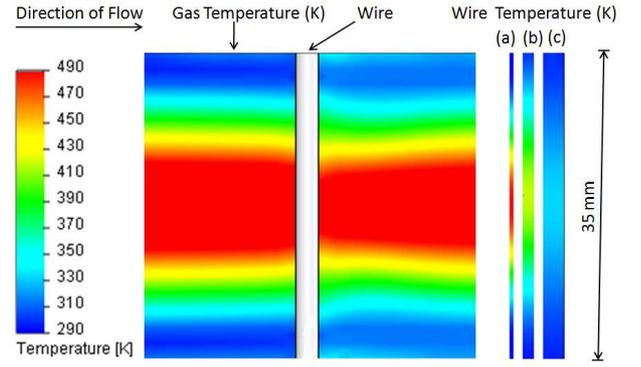
Fig. 4. CFD simulation of fine wires exposed to a steady-state temperature gradient (colour diagram).
