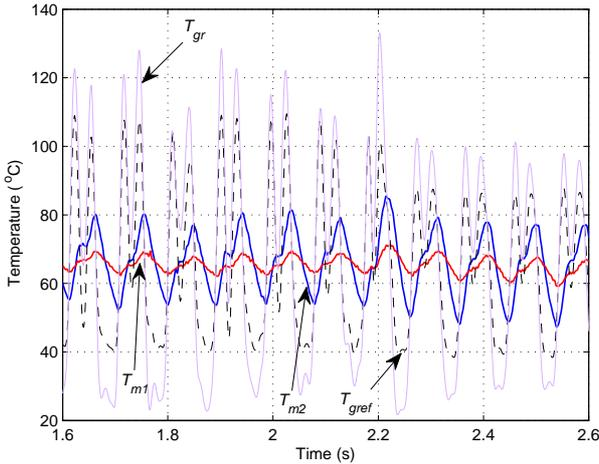
Fig. 11. Gas temperature reconstruction using  $\beta$ -GTLS PS algorithm with window size of 980 samples.
