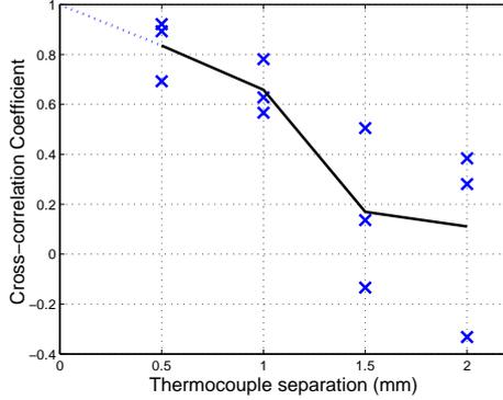
Fig. 2. Variation in correlation-coefficient between TTP thermocouple data with spacing.
