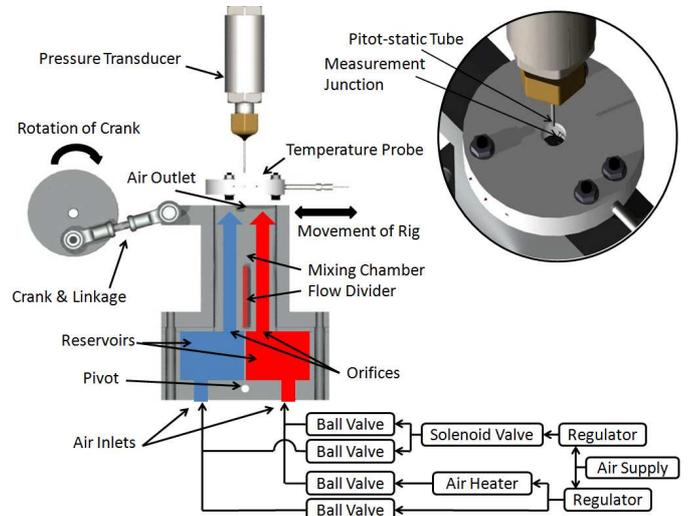
Fig. 1. Experimental test rig schematic.
