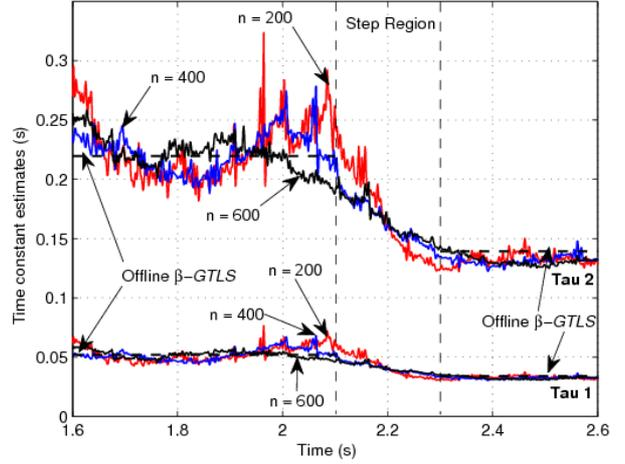
Fig. 8. Time constant estimates with varying sized data windows using  $\beta$ -GTSL PS sliding window algorithm.
