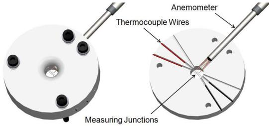
Fig. 3. Temperature measurement probe assembly.
