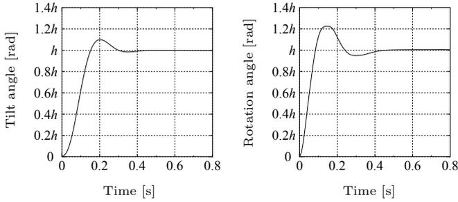
Fig. 5. Responses of the designed control systems to the step reference command  $h = 0.01745$  [rad]
