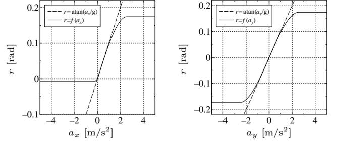
Fig. 4. Reference function (Left: reference tilt angle. Right: reference rotation angle)
