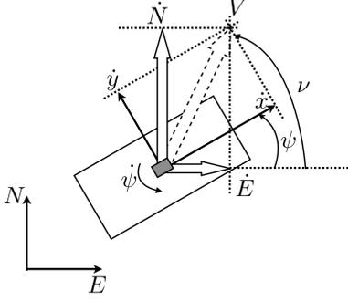
Fig. 1. Plan view showing the velocities vectors in b-frame and e-frame, also the resultant velocity.
