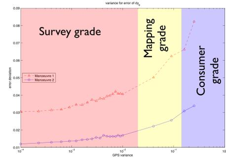
Fig. 10. Error deviation of lateral velocity over GPS variance (0.01 m/s to 0.5 m/s).  $\tau = 1$  s.
