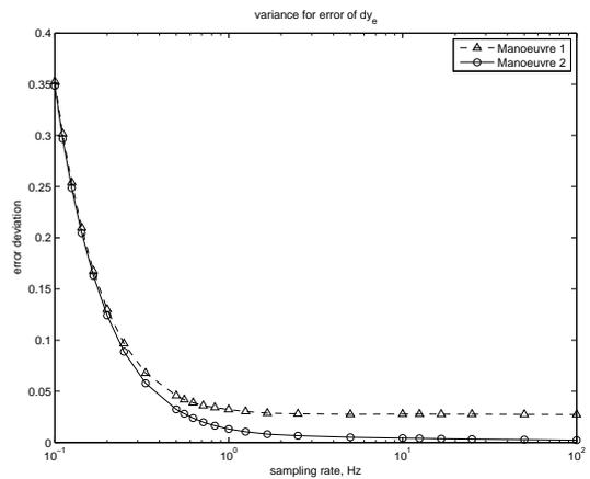
Fig. 7. Error deviation of lateral velocity over a range of GPS sampling rate (0.1 Hz to 100 Hz)
