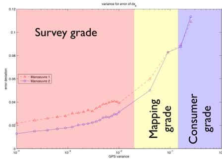
Fig. 9. Error deviation of longitudinal velocity over GPS variance (0.01 m/s to 0.5 m/s).  $\tau = 1$  s.
