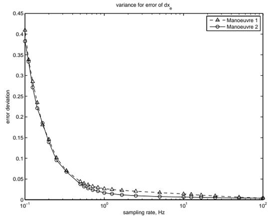
Fig. 6. Error deviation of longitudinal velocity over a range of GPS sampling rate (0.1 Hz to 100 Hz)
