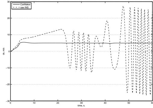
Fig. 3. Longitudinal velocity without EKF
