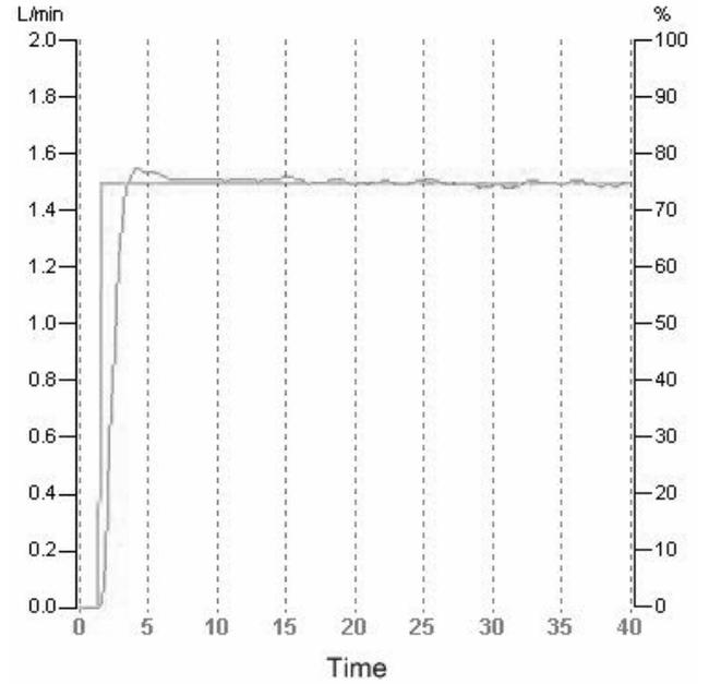
Fig. 6. Step response of the remote flow rate controller when  $T_r = 1s$ .
