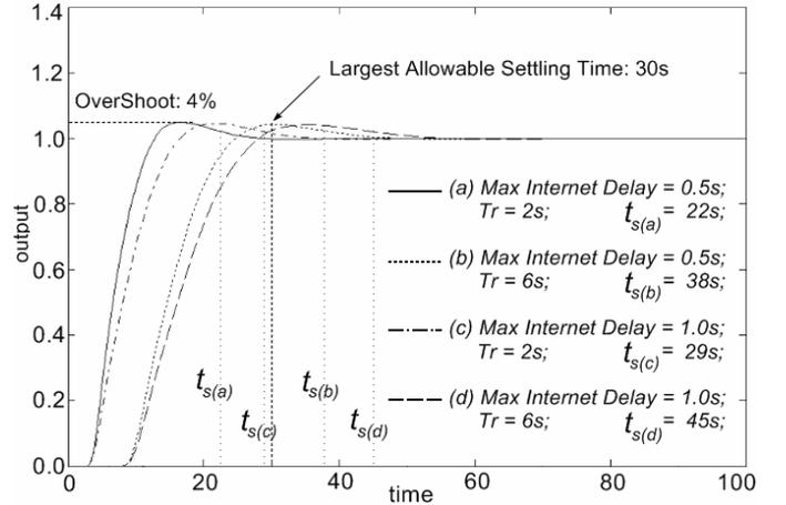
Fig. 4. Step Response in Simulation
