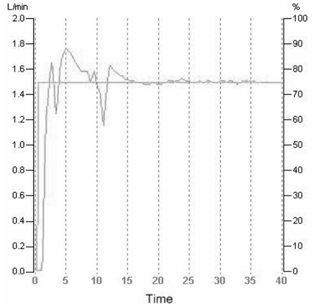
Fig. 7. Step response of the remote flow rate controller when  $T_r = 4s$ .
