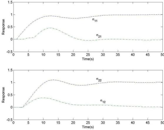
Fig. 5. Closed-Loop Response using Full Controller for the Wood and Berry Plant
