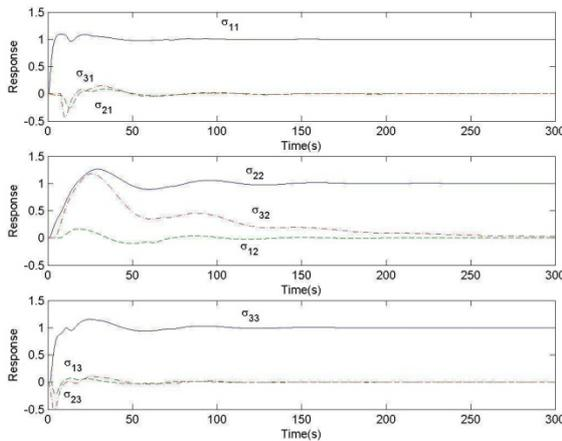
Fig. 10 Response of Tyreus Case 4 Plant to Unit Step set-point increase using Diagonal Controllers
