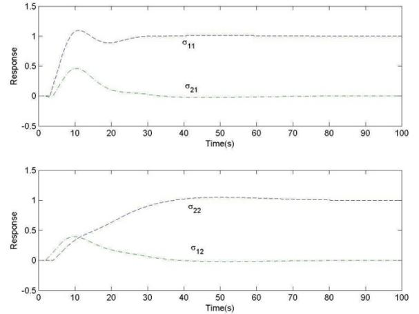
Fig. 7. Closed-loop Response of Nordfeldt and Hagglund Plant using Full Controllers
