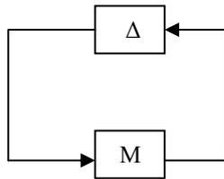
Fig. 3. Linear Fractional Transformation,  $\Delta$ - $M$  structure for studying effect of uncertainty on stability or performance.
