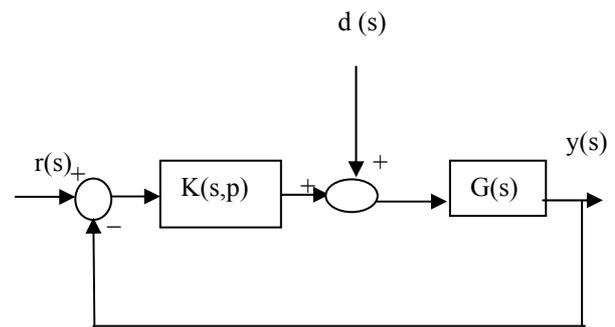
Fig. 1. Basic Control Structure Of Feedback Control
