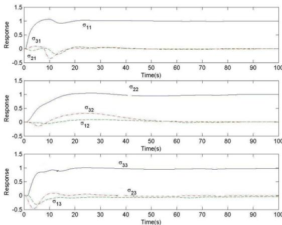
Fig. 11. Response of Tyreus Case 4 Plant to Unit Step set-point increase using Full Controllers
