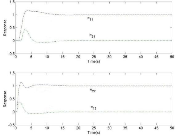
Fig. 9. Closed-Loop Response using Full Controller for the Luyben and Vinante Plant.
