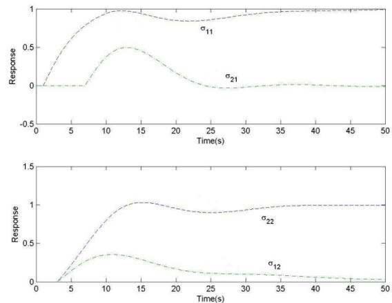
Fig. 4. Closed-Loop Response using Decentralized Controller for the Wood and Berry Plant.
