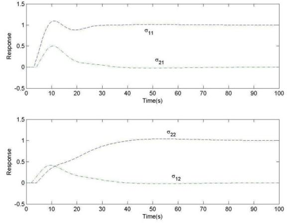
Fig. 6. Closed-Loop Response using Decentralized Controller for the Nordfeldt and Hagglund Plant.
