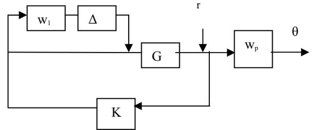
Fig. 2. Block Diagram of plant with input uncertainty and with external inputs
