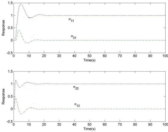
Fig. 8. Closed-Loop Response using Decentralized Controller for the Luyben and Vinante Plant.
