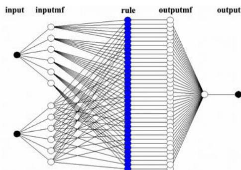
Fig. 2: ANFIS structure for modelling the TRMS
