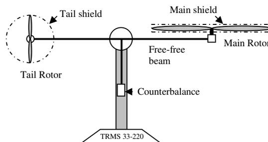
Fig. 1: Schematic diagram of the TRMS
