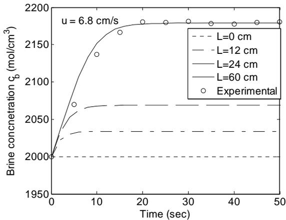
Fig.4. Dynamics of brine concentration at different axial locations inside membrane tube.
