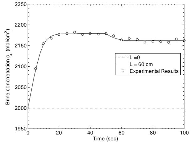
Fig.5. Dynamic response for 10 % positive step change in the feed rate.
