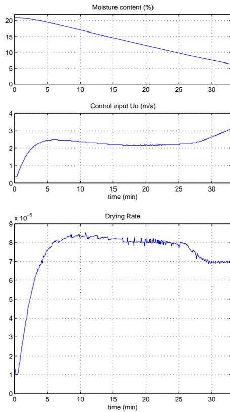
Fig. 9. Control input and moisture content using a PI controller and different drying rates (top), and drying rate (bottom).
