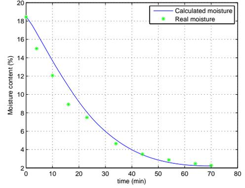
Fig. 3. Measured and calculated moisture content in a bed dryer.
