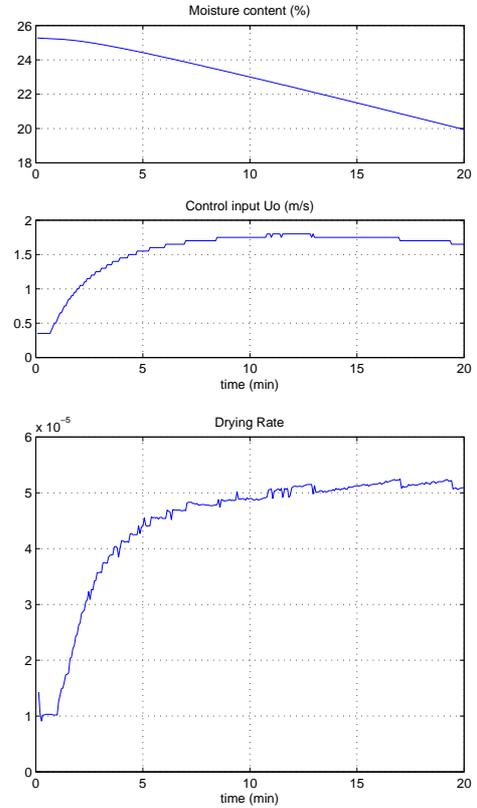
Fig. 8. Control input and moisture content using a PI controller (top), and drying rate (bottom).
