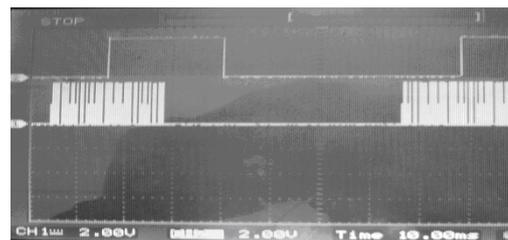
Fig.7 The experimental waveform of commutation and PWM modulation
