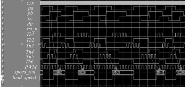
Fig.4. BLDM commutation and speed measurement module simulation waveform
