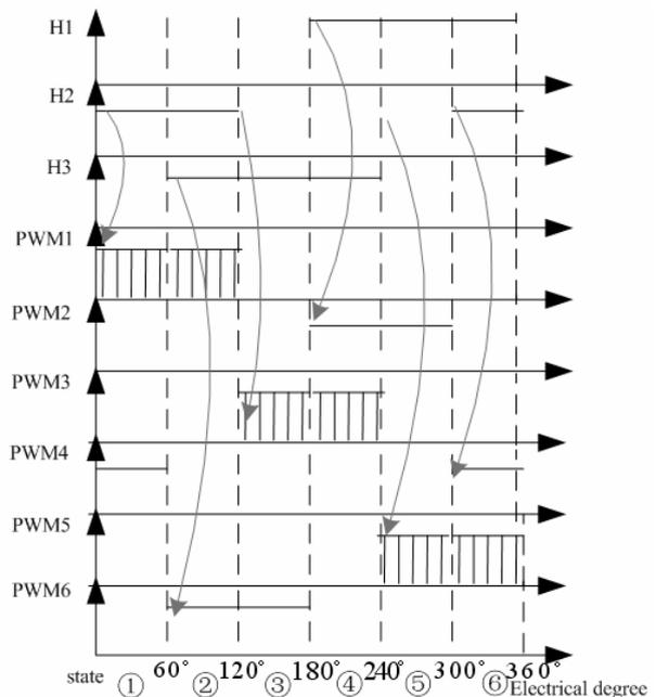
Fig.1.6-ladder waveform converted by 3-phase position signal
