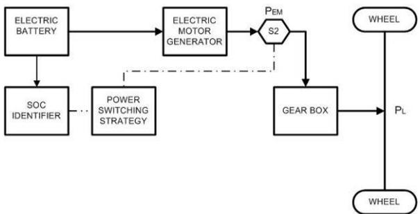
5- If the vehicle is propelled by external forces such as gravity, wind, etc or when the driver insist to break the vehicle, then the electric motor would act as a generator to capture the energy and which would effectively charge the battery. In this case the power flow would be from vehicle to the electric motor.
