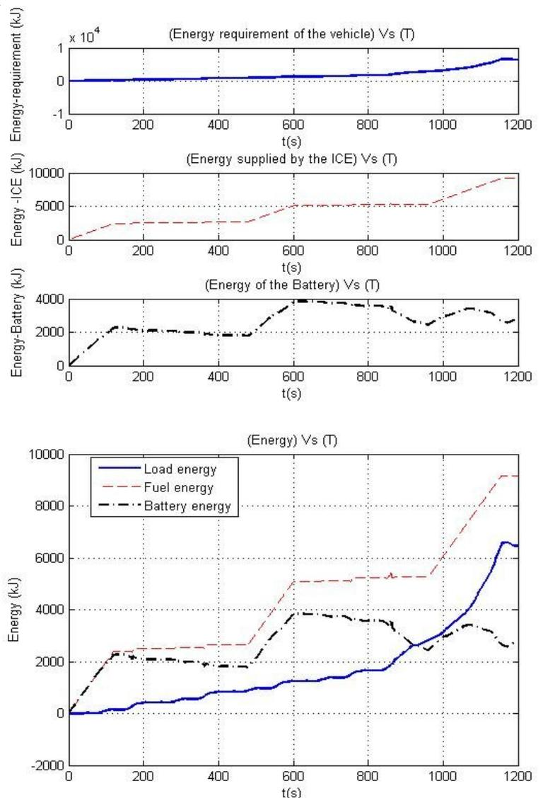
Fig. 4 simulation result shows the energy fluctuation in the dual energy sources according to the energy consumption of the vehicle.
