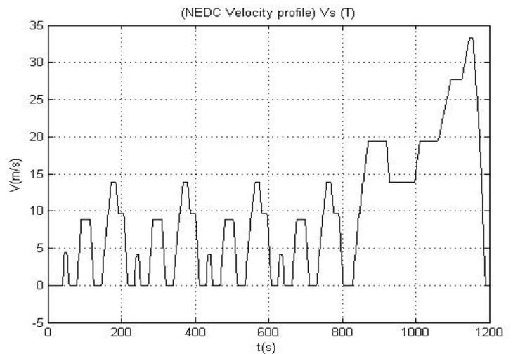
Fig. 3. the standard New European Driving Cycle (NEDC) velocity profile.
