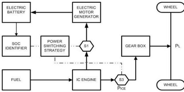
4- If the battery has the sufficient energy and if the motor is power enough to overcome the load power requirement then the electric motor alone would propel the vehicle. In this case the power flow would be from electric motor to the vehicle
