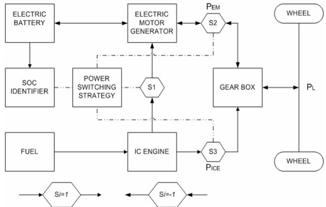
Fig. 1 Generic power flow diagram of the parallel hybrid vehicle, which includes all possible power flow directions.
