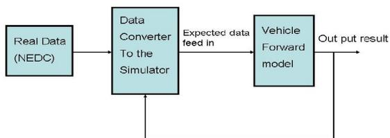
Fig. 2 the block diagram of the data converter, which feeds the standard NEDC velocity data into the vehicle forward model.
