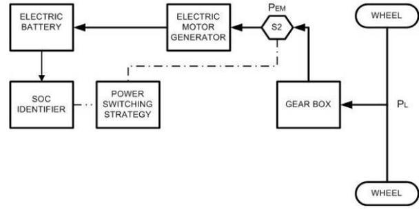
3- If the load power requirement is less than the power supplied by the IC engine, and the battery can be given more energy to accumulate, then the excess amount of power can be converted as electrical power to charge the battery. In this case the electric motor would act as generator. The power flow pattern would be as bellow.
