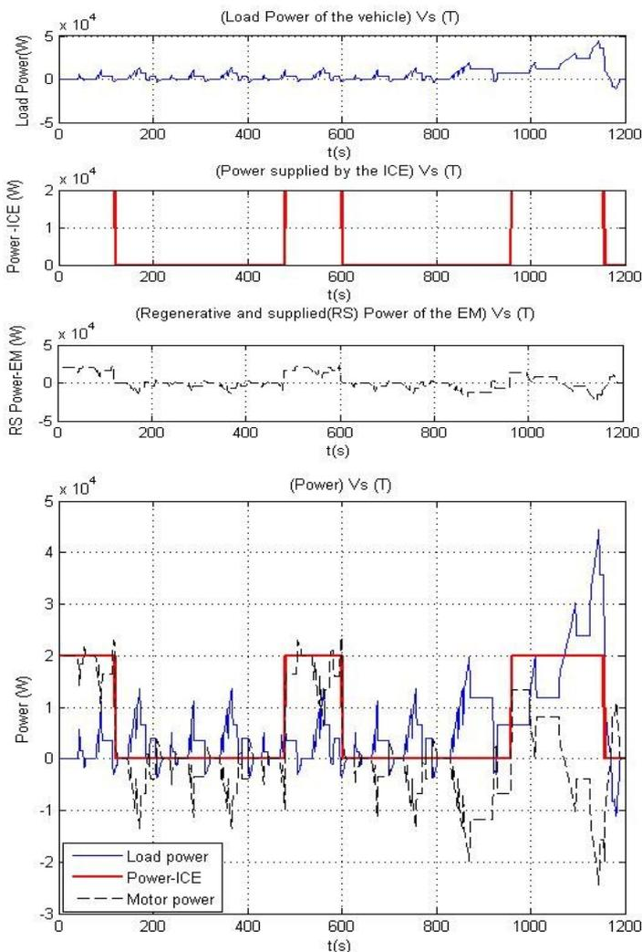
Fig. 5. Simulation results show the power demand of the vehicle and the contribution of the individual sources to supply the demand.
