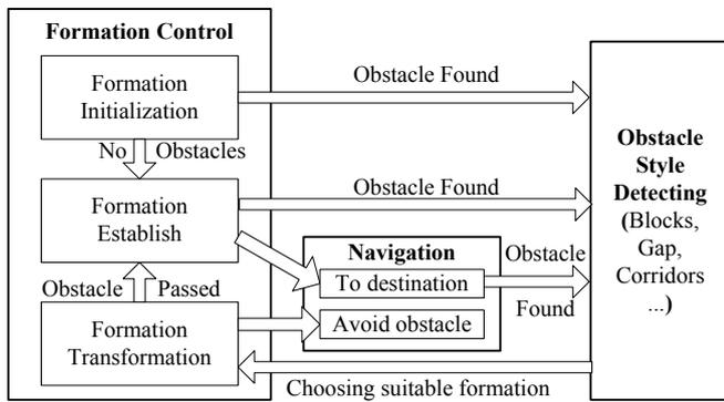
Fig.1. Overall framework of the system
