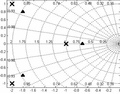
Fig. 4. The nominal poles and perturbed poles. X and  $\Delta$  points represent the perturbed poles and the nominal poles, respectively
