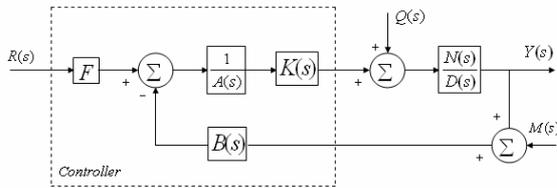
Fig. 3. CDM with PI controller K(s).
