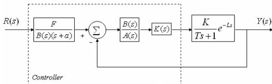
Fig. 5. The block diagram of the control system controlling FOPTD systems.
