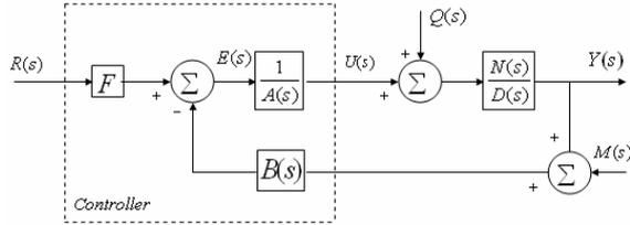
Fig. 1. The standard block diagram of CDM.
