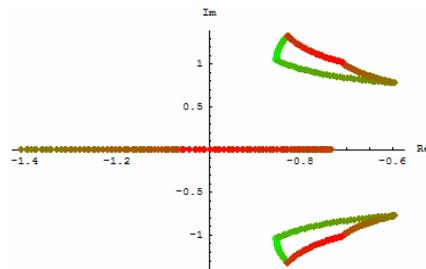
Fig. 6. Pole spread of the closed-loop system using standard CDM ( $T=2$ ,  $L=0.5$ )
