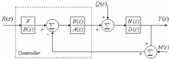
Fig. 2. Equivalent block diagram of CDM
