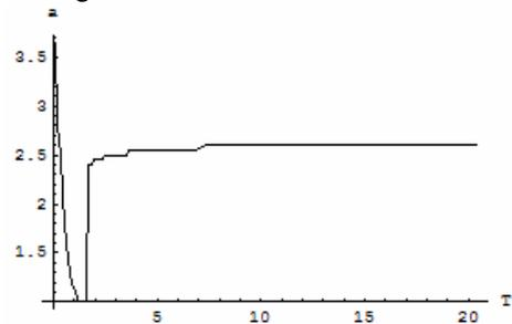
Fig. 12. The values of  $a$  parameters which make the system most robust for  $0.1 < T < 20$ . ( $L=0.5$ )
