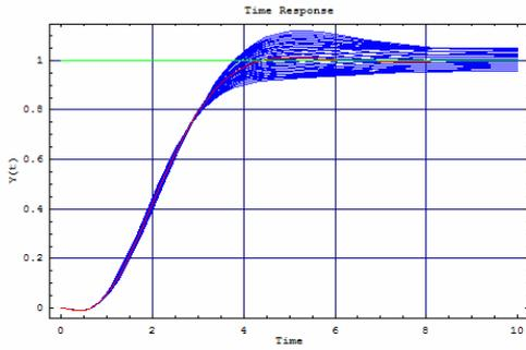
Fig. 7. Unit step response of the closed loop system using standard CDM ( $T=2$ ,  $L=0.5$ )
