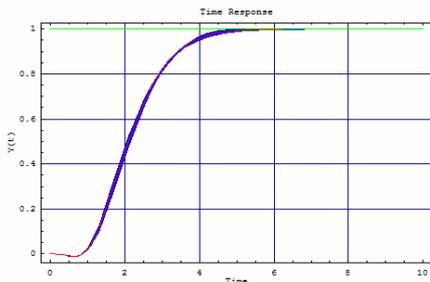
Fig. 9. for CDM-PI controller, the unit response spread of the closed loop system ( $T=2$ ,  $L=0.5$ ,  $a=1$ )
