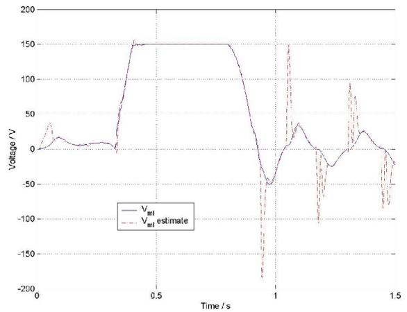
Fig. 9 – Azimuth Voltage from PWM Integrator
