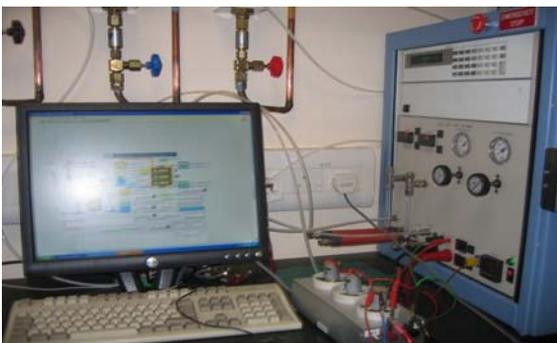
Fig.2. Fuel cell Test bench with 300-W fuel cell stack
