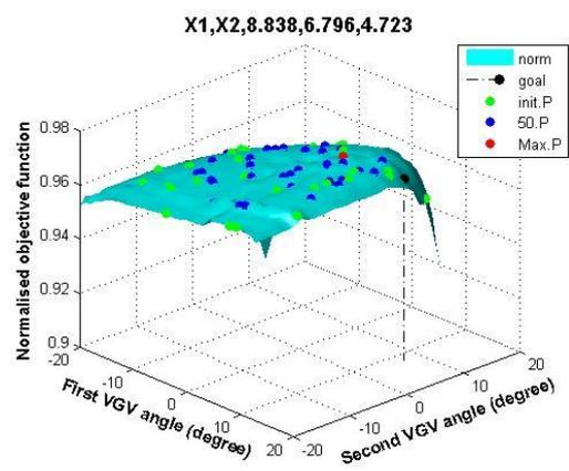
Fig. 6. 2-D VGV variation at 8000 rpm
