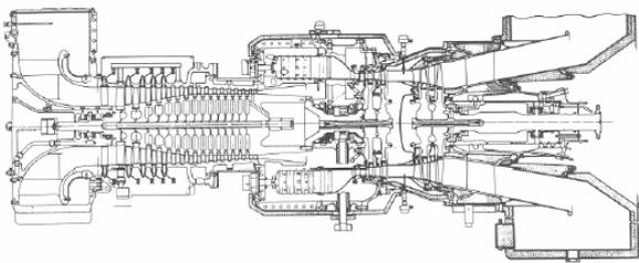
Fig.1. Schematic view of Tornado gas turbine engine
