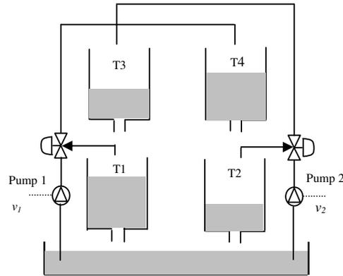
Fig.4. Schematic diagram of the quadruple-tank process
