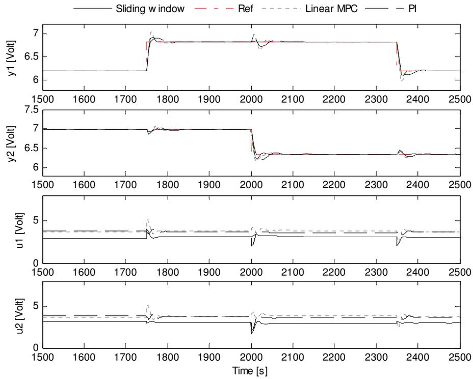
Fig.5 The comparison of control performance MP system
