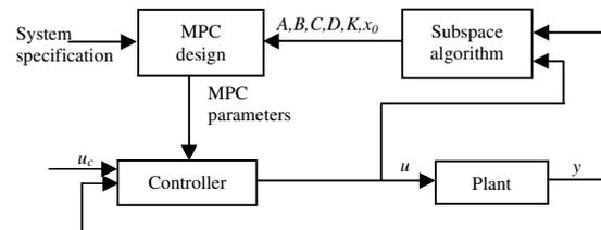
Fig.1. Indirect Adaptive Control
