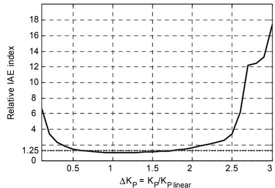
Fig. 6. Effect of the nonlinear gain variations on the relative IAE index
