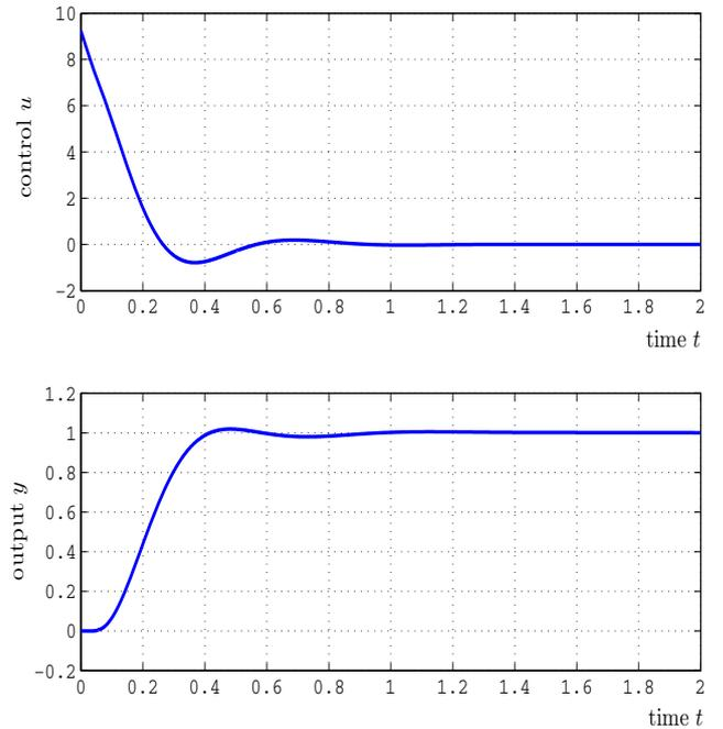
Fig. 3. Step responses of heat conduction system
