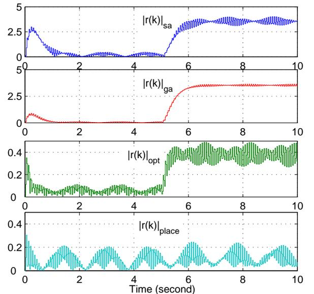
Fig. 3. Residual norms of  $K_{sa}$ ,  $K_{ga}$ ,  $K_{opt}$  and  $K_{place}$ , corresponding to the abrupt fault (28)
