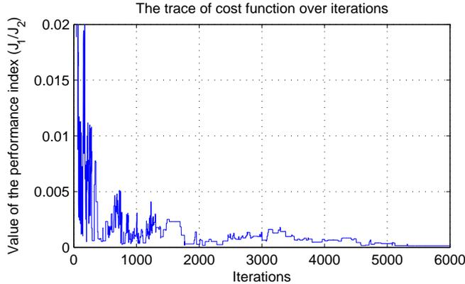
Fig. 2. Trace of the cost function values over iterations in the simulated annealing optimisation. It involves 6000 search iterations and one cost function evaluation in each iteration. In total, the number of objective function evaluation in this simulated annealing optimisation is 6000.
