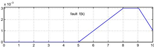
Fig. 4. The fault signal of Eq. (29).
