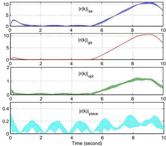
Fig. 5. Residual norms of  $K_{ga}$  (blue),  $K_{opt}$  (read),  $K_{place}$  (green), corresponding to the incipient fault (slope=0.00001)
