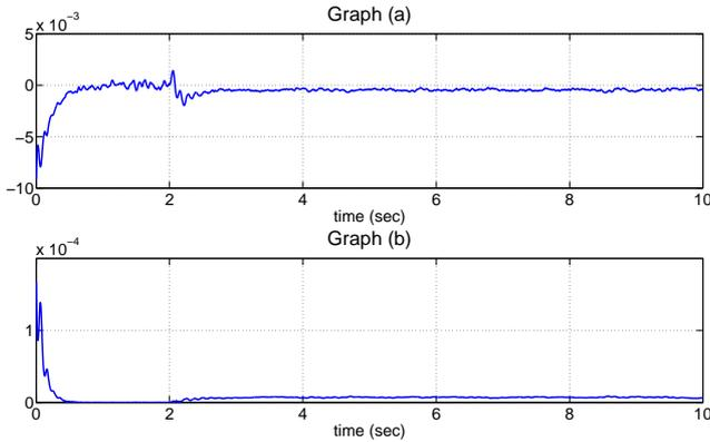
Fig. 3. Kalman-Like Result (a)residual response for leak (b) output error residual  $\hat{y} - y$
