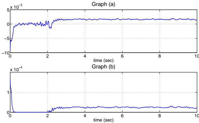
Fig. 4. High Gain Observer (a)residual response for leak (b)output error residual  $\hat{y} - y$
