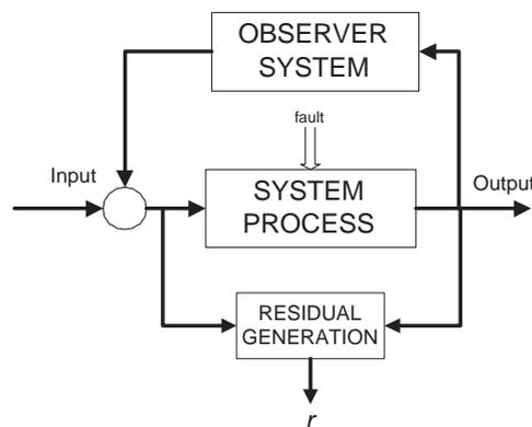
Fig. 1. Block Diagram Representation of Fault Detection Scheme via High Gain Observer Technique
