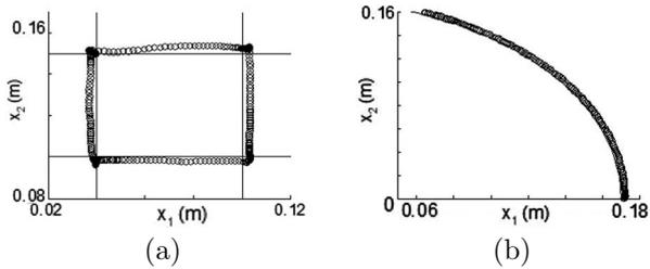
Fig. 7. Tracing a virtual shape with Controller 3. (a) Square from the inside. (b) Circle from the inside. Solid line - constraint. Marked line - experimental trajectory traced by the manipulator tip.
