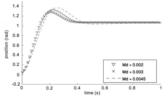
Fig. 5. Response to a unit step input torque for different desired inertias with Controller 2.  $B_d = 0.05\text{Nms/rad}$  and  $K_d = 1\text{Nm/rad}$  in each case.
