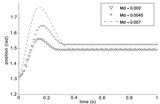
Fig. 6. Response to a unit step input torque for different desired inertias with Controller 1.  $B_d = 0.03\text{Nms/rad}$  and  $K_d = 4\text{Nm/rad}$  in each case.
