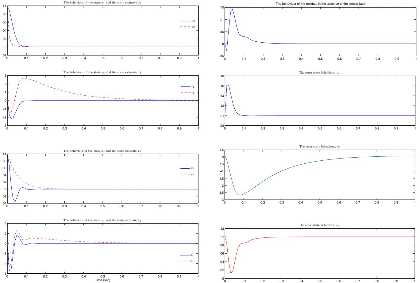
Fig. 1. The behaviour of states and their estimates for the nonlinear M-S-D system.
