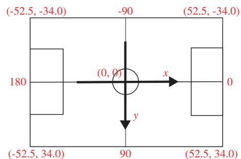
Fig. 1. The coordination systems of Robocup Soccer Simulation
