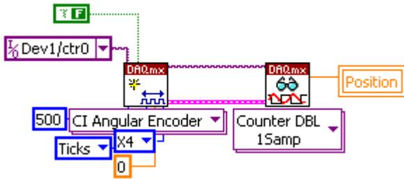
Fig 5 Software reading the encoder interface
