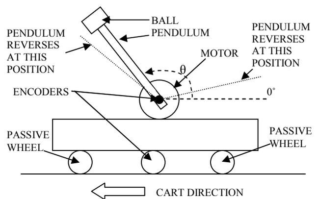
Fig 1 Schematic of the driven inverted pendulum
