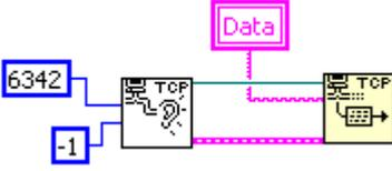
Fig 8 TCP Client program section
