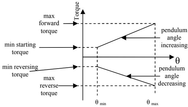
Fig 11 Torque profile
