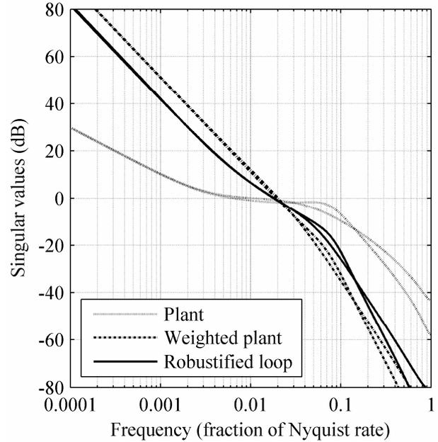
Fig. 7. Singular values (frequency response) of plant before and after weighting, and after loop robustification using  $H_\infty$  synthesis.
