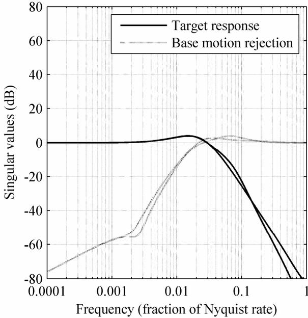
Fig. 8. Closed-loop singular values (frequency response) achieved through  $H_\infty$  loop-shaping.
