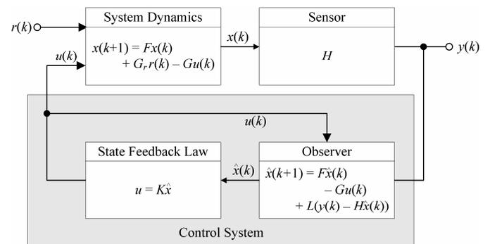
Fig. 2. State-feedback control system with an observer. The observer attempts to estimate the state of the system dynamics; the estimated state is used to approximate a state feedback control law.
