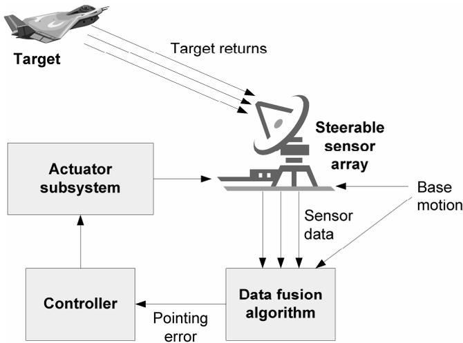
Fig. 1. Tracker schematic. This diagram gives a high-level conceptual illustration of the tracker configuration.
