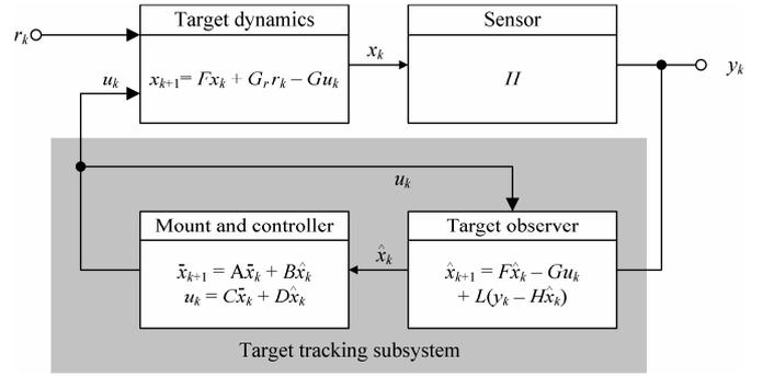
Fig. 5. Separation of tracking and steering (sec. 3.2).
