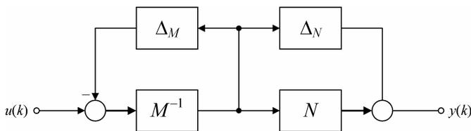
Fig. 3. Normalized right-coprime factorization. This structure can be used to represent a system with uncertain dynamics: the delta blocks are perturbations to the nominal system.
