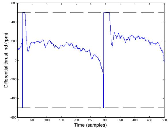
Fig. 9. Differential thrust produced by the standard LQG autopilot
