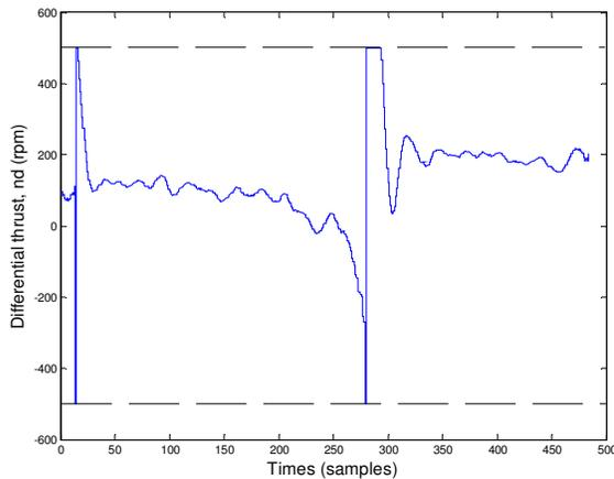
Fig. 10. Differential thrust produced by the fuzzy LQG autopilot
