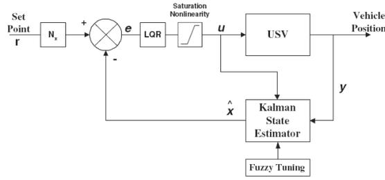
Fig. 5. Fuzzy LQG controller block diagram
