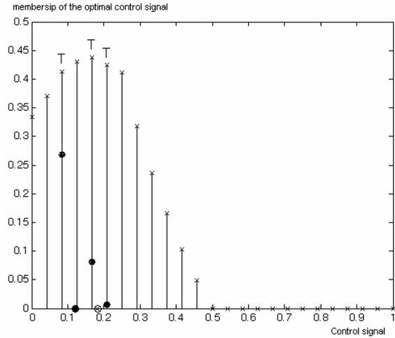
Fig. 5 Membership of the optimal control signal when the model has been partially trained
