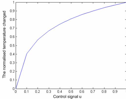
Fig. 3 Example non-linearity of a cooling coil
