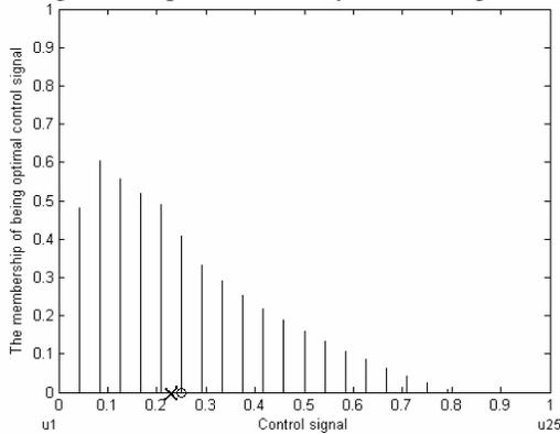
Fig. 4 Membership of the optimal control signal
