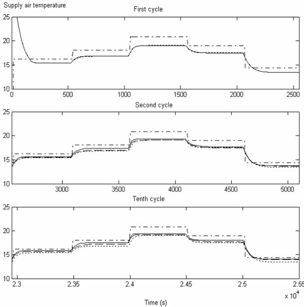
Fig. 8 Supply air temperatures when the model has been trained on-line to track repeated step changes
