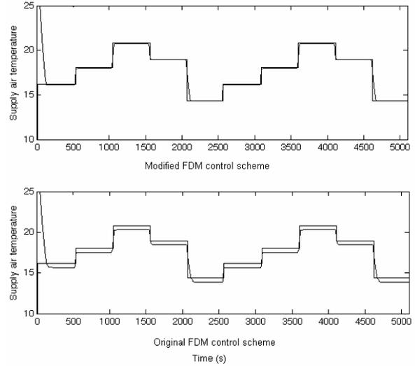
Fig. 7 Control of the supply air temperature using a fully trained “ideal” model
