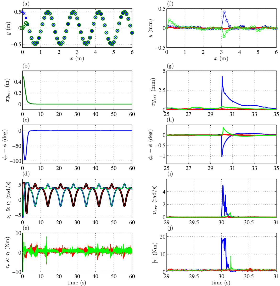
Fig. 4. (a): reference (blue) & actual (green) trajectories; (b): position error; (c): orientation error; (d): velocities - right (red), left (green) & their references (black & blue respectively); (e): torques - right (green), left (red); (f) to (j): comparative results - HCE (blue), Cautious (green), Dual (red).
