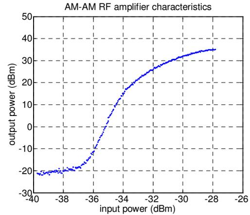
Fig. 4. AM/AM characteristics of the given amplifier
