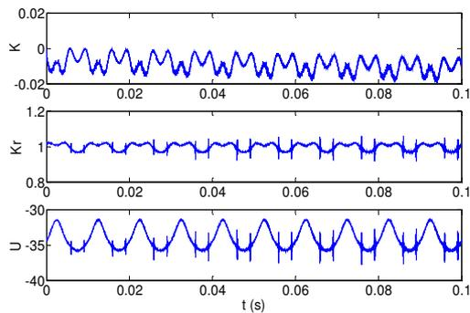
Fig. 10.  $K$ ,  $K_r$ ,  $u$  are feed-forward, feedback parameter and control signal respectively
