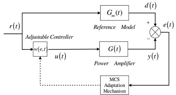
Fig. 2. Typical model reference adaptive system structure for linearisation of power amplifiers
