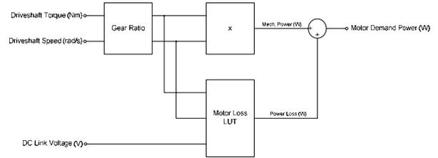
Fig. 3 Model for the motor demand power
