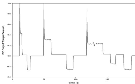
Fig. 11. PID controller response over ECE cycle
