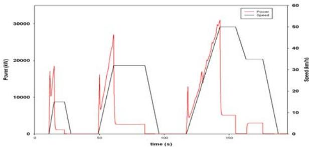
Fig. 9. Drive Power and vehicle speed for ECE Cycle
