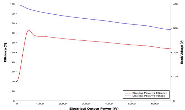
Fig. 8. Stack voltage response to load changes
