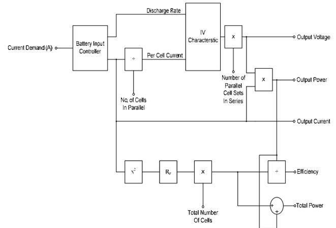
Fig. 6. Model of the battery pack
