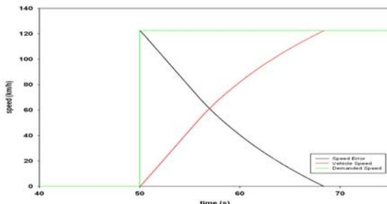
Fig. 10. Vehicle step response to full speed demand
