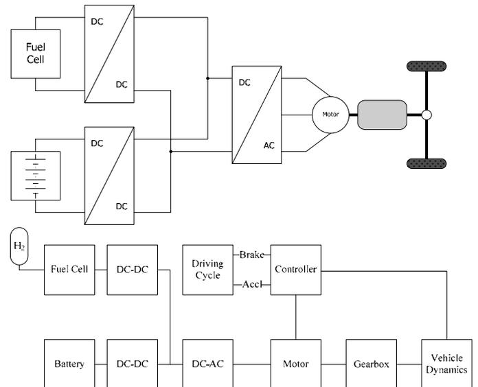
Fig. 1. Top: Topology of a hybrid electric fuel cell power drive train. Bottom: Equivalent schematic of simulation model
