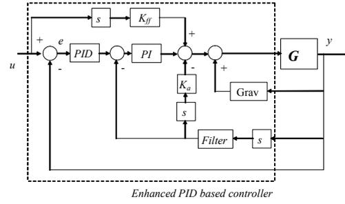
Fig. 3. Structure of the enhanced PID based control.
