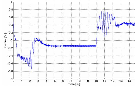
Fig. 9. Control signal with anti-chattering algorithm.
