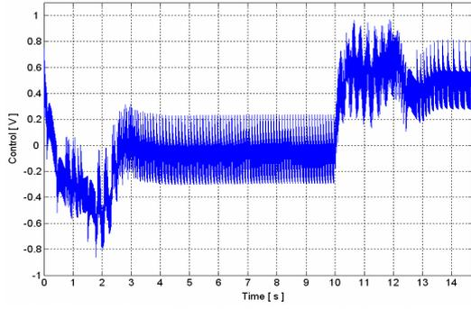
Fig. 8. Chattering effect in the control signal.
