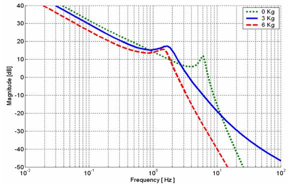
Fig. 2. Linear transfer functions for 0, 3 and 6 kg.
