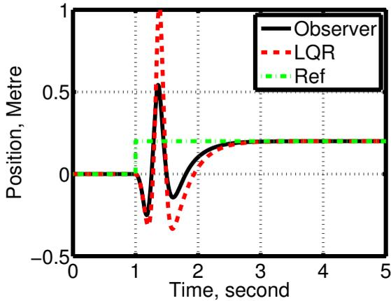
Fig. 6. Comparison of step response of cart for LQR and multiple-observer based control under poor channel conditions
