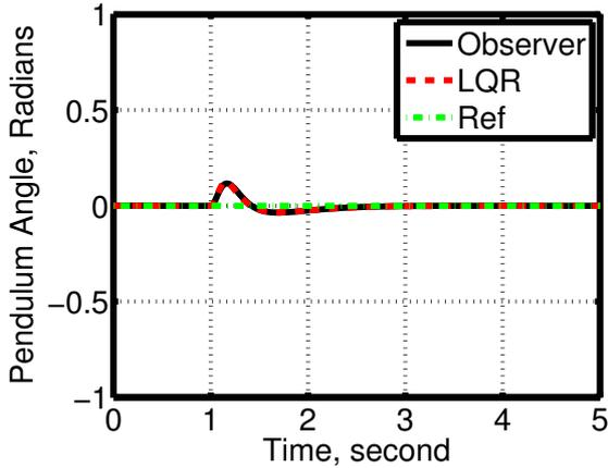
Fig. 5. Comparison of step response of pendulum angle for LQR and multiple-observer based control under good channel conditions
