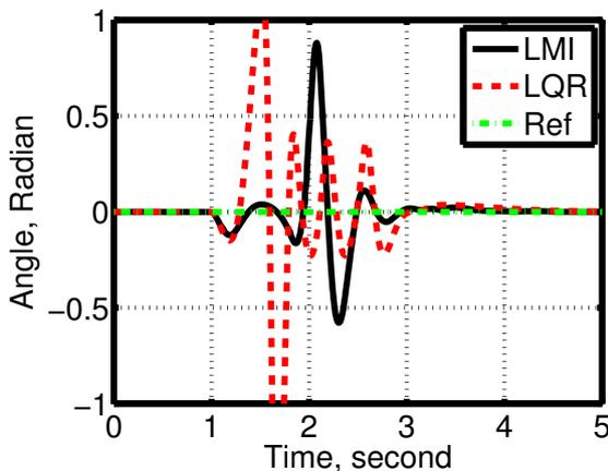
Fig. 11. Comparison of pendulum angle during step response for LQR and multiple-observer based control WNCs experiments under poor channel conditions
