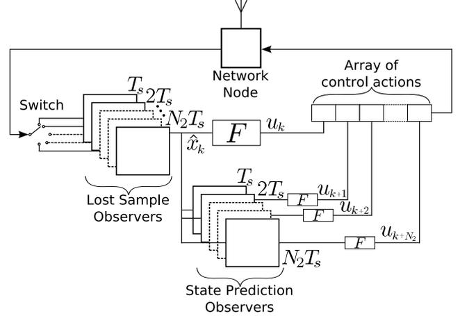
Fig. 2. Multi-observer based control for WNCS
