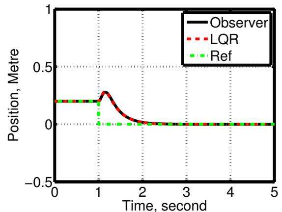
Fig. 4. Comparison of step response of cart for LQR and multiple-observer based control under good channel conditions
