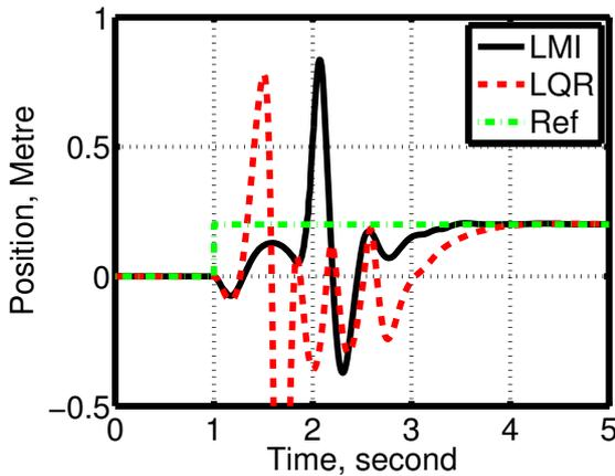
Fig. 10. Comparison of step response of cart for LQR and multiple-observer based control WNCs experiments under poor channel conditions
