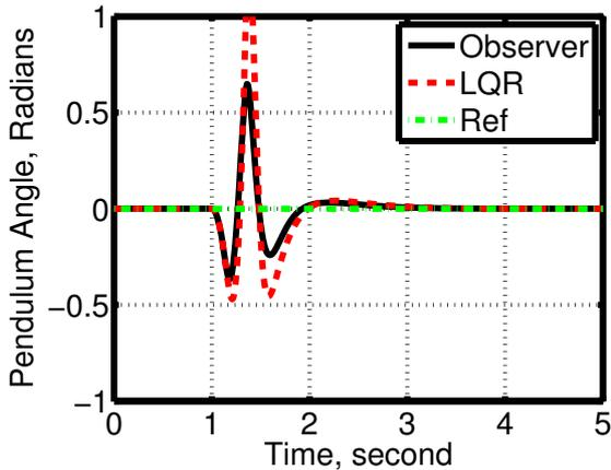
Fig. 7. Comparison of pendulum angle during step response for LQR and multiple-observer based control under poor channel conditions
