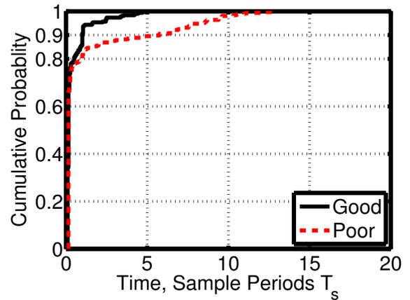
Fig. 3. Cumulative distribution functions for experimentally measured  $\tau_{sa}$  variable time delay. Good channel conditions 90% of delays below  $T_s$ , poor channel conditions 90% of delays below  $6T_s$
