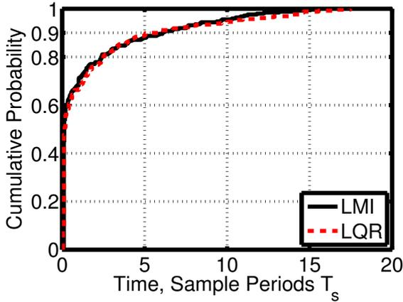
Fig. 9. Cumulative Distribution Functions for delays in WNCs experiments with multiple-observer and LQR based control - poor channel conditions (90% of Delays below  $7T_s$ )
