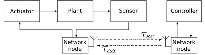
Fig. 1. Wireless Network Control System
