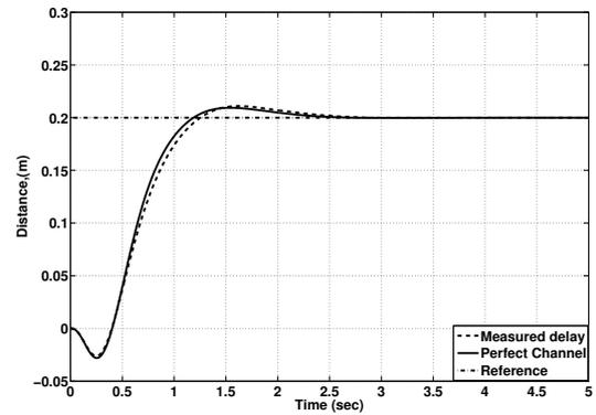
Fig. 5. Variation in average cart position step response under DMC control and delay compensation, for the measured random delay ( $ITAE_n = 1.9 \times 10^{-3}$ ).
