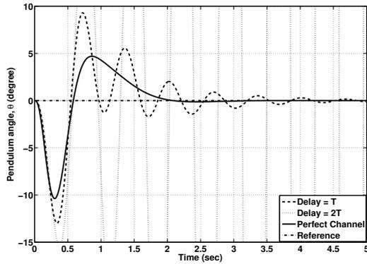
Fig. 3. Comparison of pendulum angle regulation for DMC between perfect channel, one with  $T$  delay ( $ITAE = 1 \times 10^{-2}$ ) and one with  $2T$  delay ( $ITAE = 5.9$ ).
