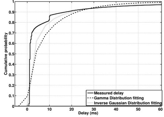
Fig. 4. Measured CDF of delay with fitted Gamma and Inverse Gaussian distributions.
