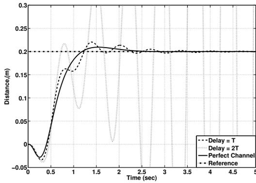
Fig. 2. Comparison of cart position step responses for DMC between perfect channel, one with  $T$  delay ( $ITAE = 2.6 \times 10^{-4}$ ) and one with  $2T$  delay ( $ITAE = 1.6 \times 10^{-1}$ ).
