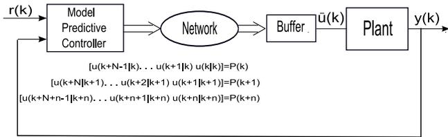
Fig. 1. The networked predictive control system with communication delay in the forward channel.
