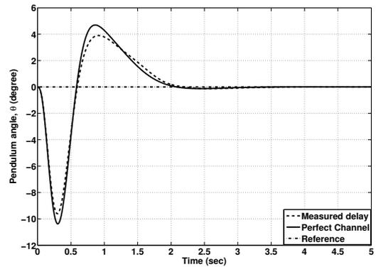
Fig. 6. Variation in average pendulum angle regulation for DMC control and delay compensation, for the measured random delay ( $ITAE_n = 1.5 \times 10^{-1}$ ).
