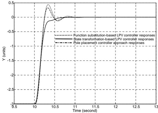
Fig. 4. Nonlinear step response from -3 to 0 with original nonlinear plant.
