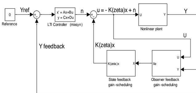
Fig. 6. Pole placement controller design.
