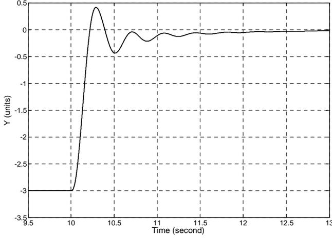
Fig. 3. Nonlinear step response from -3 to 0 of new Jacobian-based LPV controller with original nonlinear plant.
