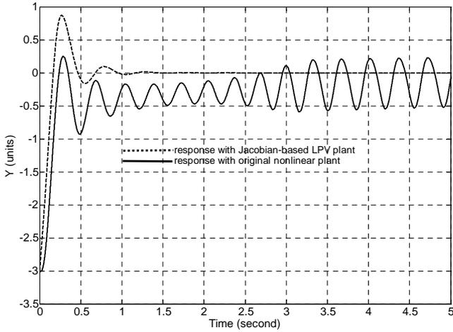
Fig. 1. Nonlinear step response from -3 to 0 of Jacobian-based LPV controller.
