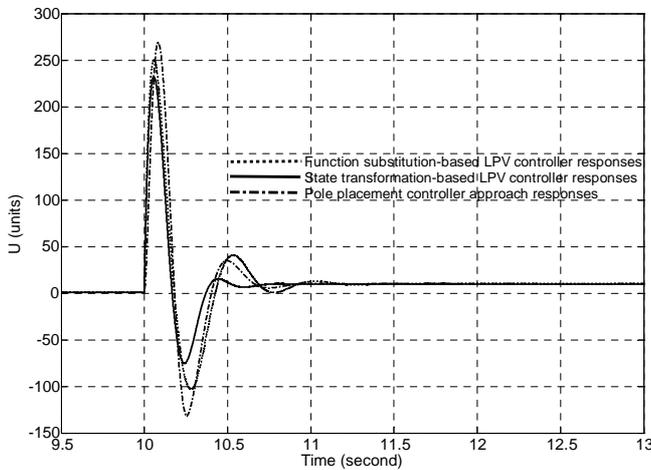
Fig. 5. Control input to original nonlinear plant.
