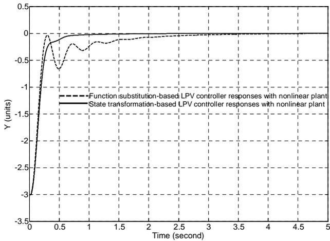
Fig. 2. Nonlinear step response from -3 to 0 of function substitution-based and state transformation-based LPV controllers.
