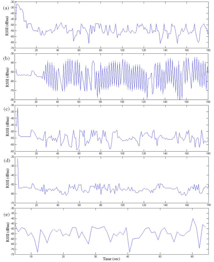
Fig. 8. Mobile Node Power Control
