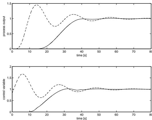
Fig. 9. Process output and control variable with the determined command input (solid line) and with a step set-point signal (dashed line) for the simulation example 2 ( $\tau = 25$ ).
