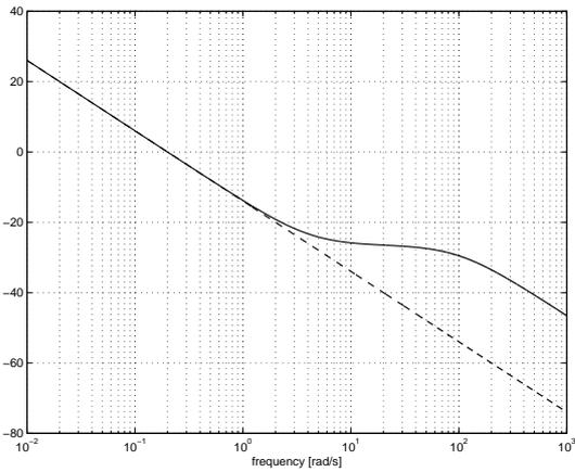
Fig. 3. Bode plot of the resulting open-loop system  $C(s)P(s)$  (solid line) and of the target function  $\bar{L}(s)$  (dashed line) for the simulation example 1 ( $\tau = 25$ ).
