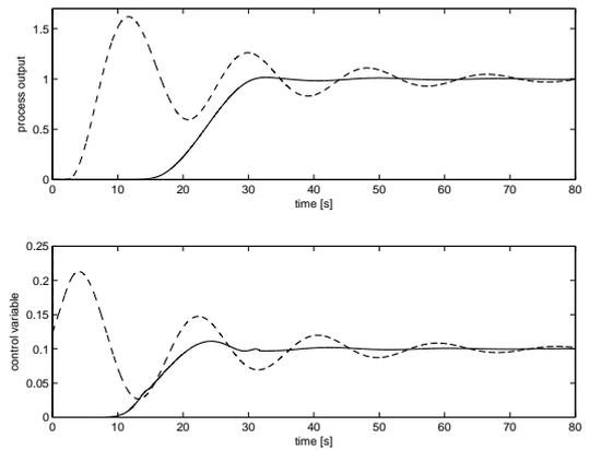
Fig. 7. Process output and control variable with the determined command input (solid line) and with a step set-point signal (dashed line) for the simulation example 1 ( $\tau = 17$ ).
