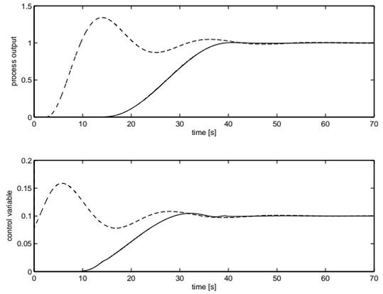
Fig. 5. Process output and control variable with the determined command input (solid line) and with a step set-point signal (dashed line) for the simulation example 1 ( $\tau = 25$ ).
