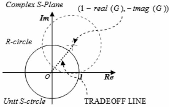
Fig. 2: Geometry of  $S$  and  $R$
