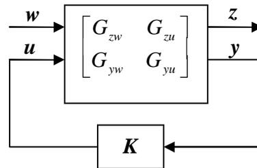
Fig. 1: The general control configuration involves four different kinds of signals: exogenous input  $w$ , controlled input  $u$ , performance  $z$  and measurement  $y$ .  $K$  is a stabilizing controller.
