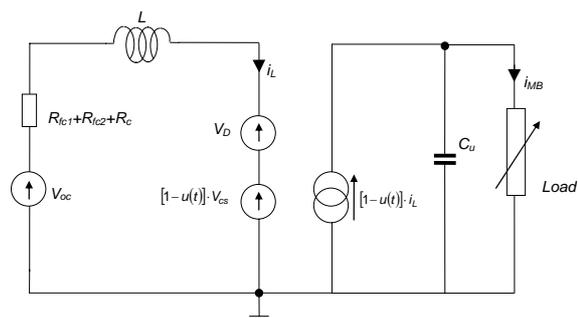
Fig. 2. Equivalent circuit diagram for the floating bus architecture model (low bandwidth model)
