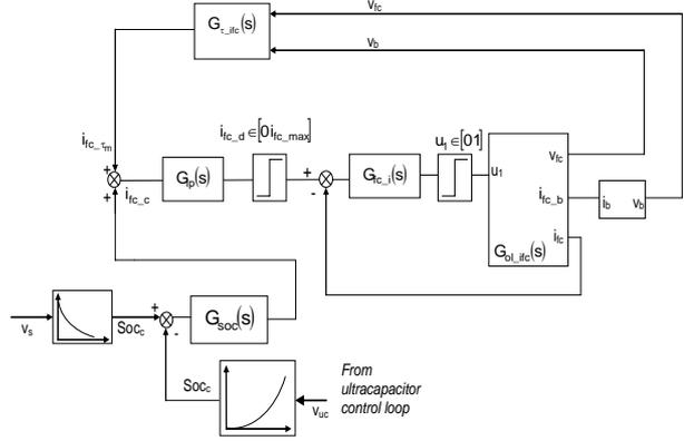
Fig. 6. Fuel cell control loop for the HEV electrical architecture
