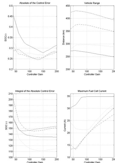
Fig. 8. Performance sensitivity of the SOC control loop to variations in the controller gain
