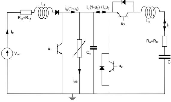
Fig. 5. Equivalent circuit diagram for the fixed bus architecture model (low bandwidth model)
