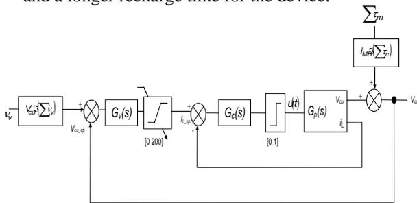
Fig. 3. High voltage bus management strategy for the floating bus architecture
