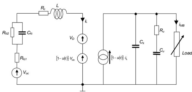
Fig. 1. Equivalent circuit diagram for the floating bus architecture model (high bandwidth model)
