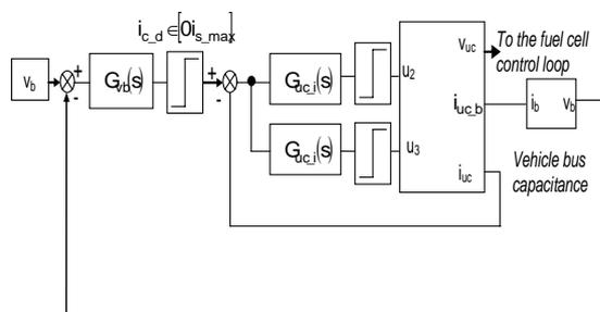
Fig. 7. Ultracapacitor control loop for the HEV electrical architecture
