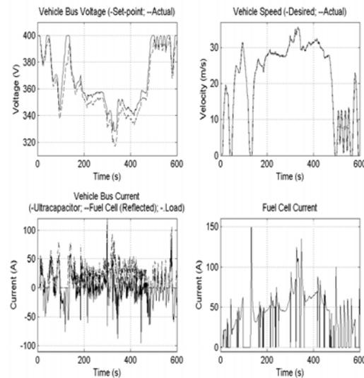
Fig. 4. Performance of the high voltage bus management system over US06
