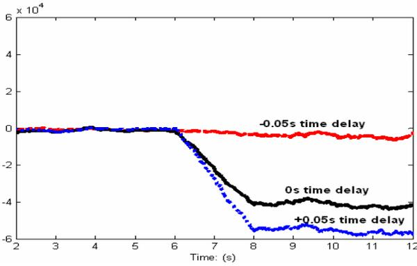
Fig. 10. Running CCF value with bounce and roll accelerations
