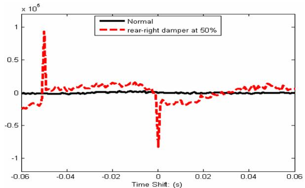
Fig 8. CCF value between pitch and roll accelerations
