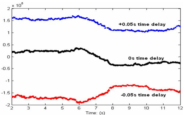
Fig 9. Running CCF value with bounce and pitch accelerations
