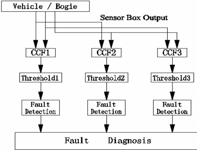
Fig 2. Proposed Fault Detection and Diagnosis Scheme
