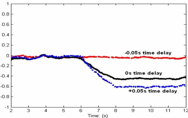
Fig 11. CCF coefficient between bounce and roll accelerations
