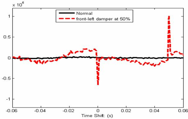
Fig 5. CCF between pitch and roll accelerations
