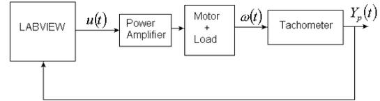
Fig. 7. DC motor speed control
