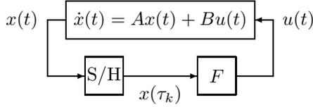
Fig. 1. Feedback control with aperiodic sample-and-hold circuits
