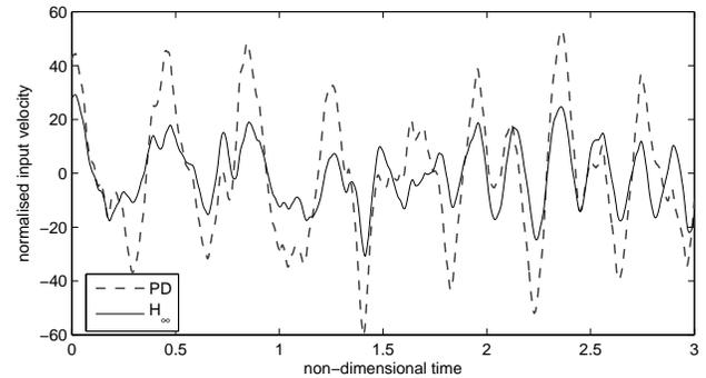
Fig. 4. Comparing control input (flap deflection) velocity for  $\mathcal{H}_\infty$  and PD controllers.
