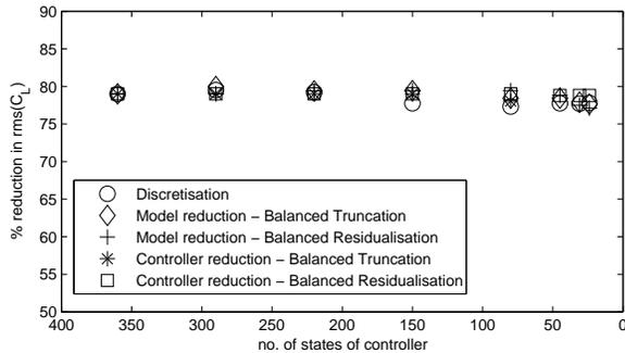
Fig. 3. Comparison of performance using  $\mathcal{H}_\infty$  controllers of decreasing sizes synthesized from spatial discretisation and different model reduction techniques.
