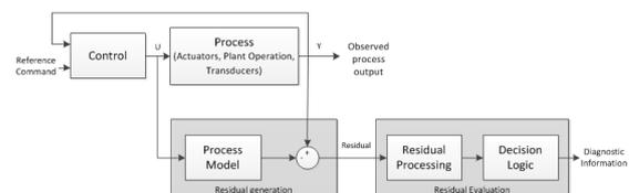
Fig. 2. Schematic of the condition monitoring scheme
